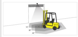
Vehicle approaches: Vehicle-detection relay is activated. Door opens.
