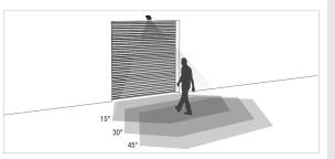
Person approaches: Vehicle-detection relay is not activated. Door remains closed.
