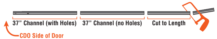
IMAGE 3: Cut and arrange the mounting channel sections
