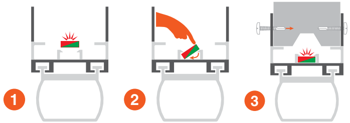
IMAGE 5: Installing the LED strip and the Aries mounting channel onto a bottom door section
